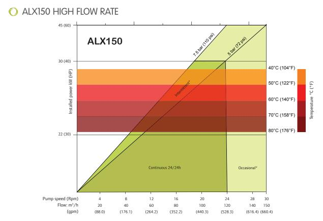
1 rpm = 5.000 m<sup>3</sup>/hr = 22.0143 gpm 1 rev = 83.3333 L = 22.0143 gal
